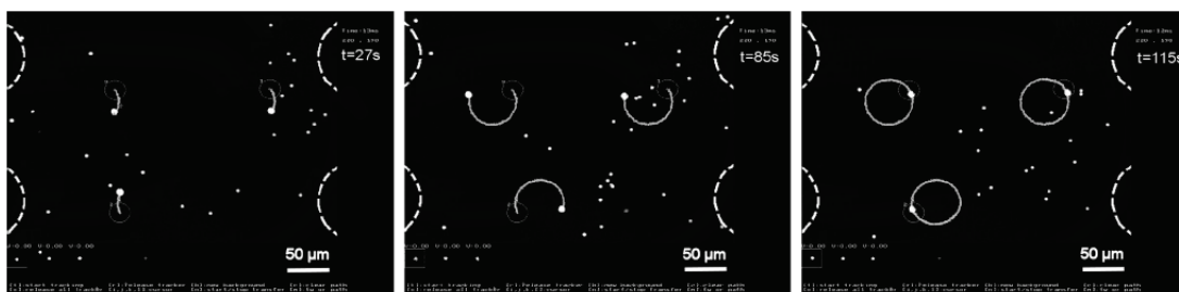
Figure 27: Steering of 3 fluorescent beads (2.2 \mu\text{m} diameter, Duke Scientific) with large surface charge (electrophoretic mobility of -92.0 \pm 15.6 \times 10^{-9} \text{ m}^2 \text{ V}^{-1} \text{ s}^{-1} ) around 3 circles. The electroosmotic mobility of my PDMS devices is u = 36.5 \pm 3.6 \times 10^{-9} \text{ m}^2 \text{ V}^{-1} \text{ s}^{-1} . In the experiment, the fluorescent beads appear as small green dots on a black background and the device geometry, which does not fluoresce, is not visible. Here, the white dots are the beads (enlarged), the blue curves are the actual trajectories that the target beads have traced out (overlaid), and the dashed white curves (also overlaid) show the geometry of the channels and the particle control chamber. Snapshots are shown at three time steps. The three beads are being steered to within an accuracy of one pixel (corresponding to less than 1 \mu\text{m} ). The desired paths are not shown because, at this image resolution, they would perfectly underlay the actual paths.
