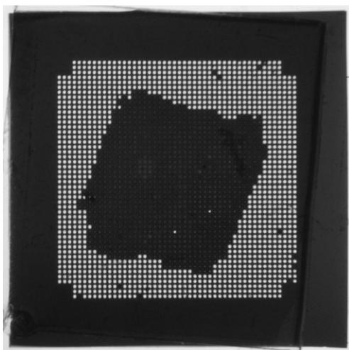
**Fig. 5** Silicon substrate having a 1 cm<sup>2</sup> area with 100 μm diameter holes spaced 100 μm apart. The surface was pretreated with BSA and spotted with water containing food dye for visualization (dark area in center). The wells filled completely by capillary action.
