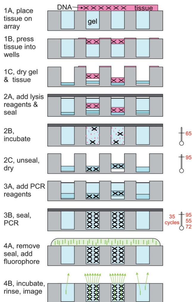
**Fig. 2** Experimental protocol used to demonstrate the 2D-PCR concept. Tissue is transferred into wells, isolated, and lysed to extract the genomic DNA (represented by “x”s). PCR is performed to amplify the target DNA, and the targets are visualized with fluorescent dye (indicated by vertical lines “|”).
