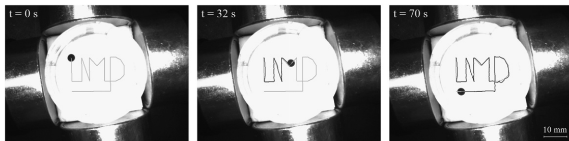
Fig. 7. Attempted control of a large 150 \mu\text{L} (3.3 mm radius) ferrofluid droplet. As soon as magnetic control is turned on, the droplet breaks up into multiple smaller droplets. This droplet was too big to control.
